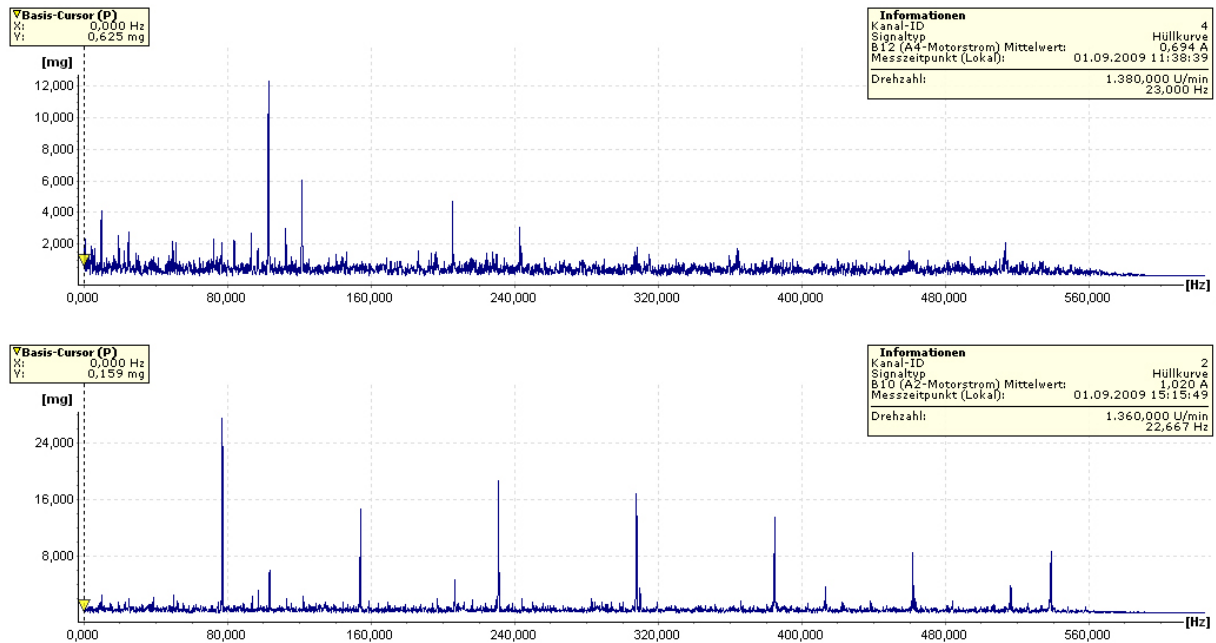
Figure 10 - Vibration analysis of roll conveyor drives
