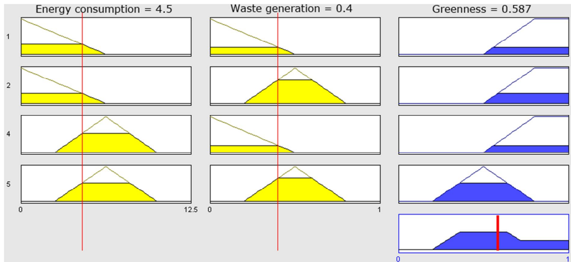
Figure 2: Evaluation of the KPI Greenness using Matlab
