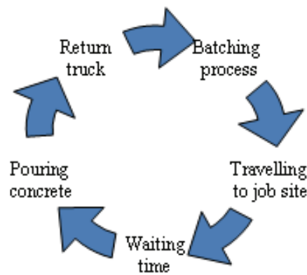
Figure 1: Ready mixed concrete delivery process
